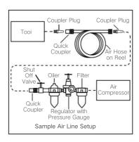
4. Connect a regulator valve, an in-line shut off valve and a 1/4" NPT air hose to the Quick Coupler (76) (all sold separately). The air hose must be long enough to reach the work area with enough extra length to allow free movement while working.
