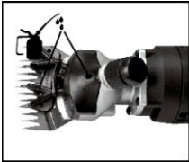
Fig. 1 (Lubricant Oiling from the Hole on the Head Shell) (Hole 1-fixed position; Hole 2 Top)
